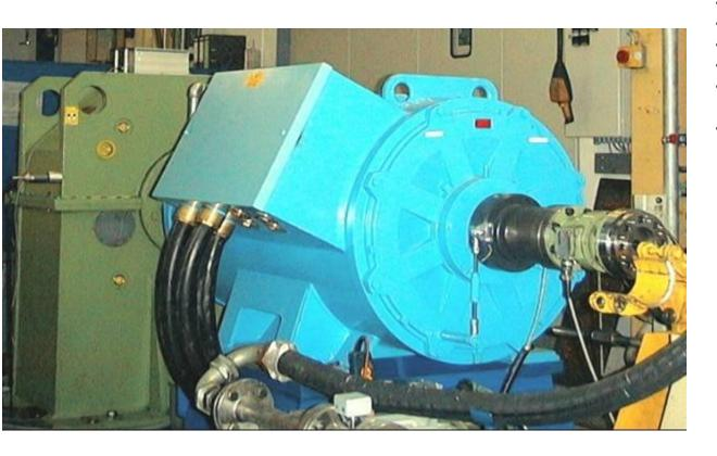
Type: MKH445L04 Power: 630 kW Voltage: 690 V
