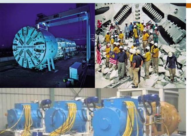
Type: MKH563K10 Power: 1100 kW Voltage: 690 V
